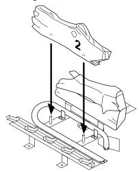
Figure 52 - Installing Log No. 2
